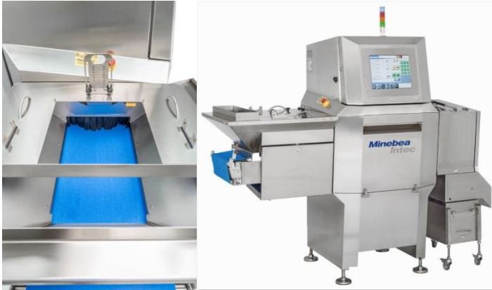
Bulk goods like nuts, smaller fruits, coffee and seeds are reliably inspected and foreign bodies eliminated
