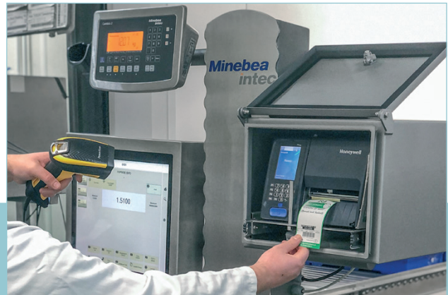
The weigh price labeller WPL-S featuring touch screen, scanner and printer
