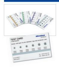
X-ray detectors can distinguish between different contaminants; therefore, we also supply multi-cards in addition to single cards. In these, up to five different ball diameters are contained in one test card.
