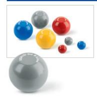
Test balls are particularly suitable for verifying metal detectors in tubular and fall-shaft systems within the conveyor tube. Depending on the diameter of the metal sphere, the diameter of the reference block is 13 mm or 30 mm. The metal spheres contained in it range in size from 0.35 mm to 5.0 mm.
