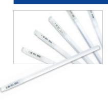
On some tube transport systems, it is not possible to place inspection and testing equipment within the product flow. To nevertheless enable a function test of the product separation, a test rod can be inserted between conveyor tube and metal detector. The test rods are made of Plexiglas. Their bendability also allows validation in angled installation scenarios.
