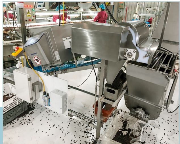
All ejected products are removed from the product stream by means of the two-way diverter flap
