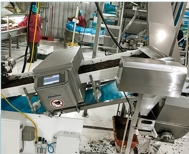
Mounted on the inclined motorization system, the metal detector is a space saving solution
