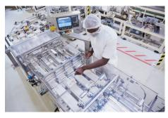
With the new WZED load cell with electromagnetic force compensation from Minebea Intec, our checkweigher models receive a turbo upgrade: the new load cell with digital controller have received MID approval in the legal-for-trade range for belt speeds of up to 3 metres per second – this means up to 600 pieces per minute. The upgrade package contains many more features that pay
