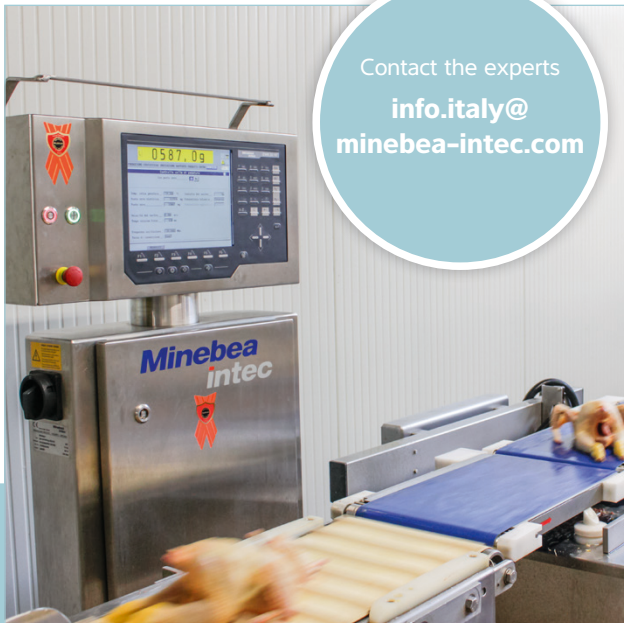
The fully cladded weighing and sorting system EWK 3010 ensures a standard throughput of over 100 pieces per minute
