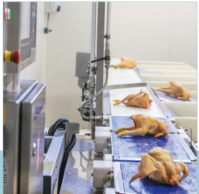
The six sorting points are defined every 50 grams, so that the poultry is precisely sorted
