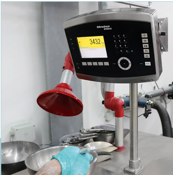
Precise weighing of pigments and additives is achieved using the bench scale. An extraction system ensures that the application is free of dust at all times
