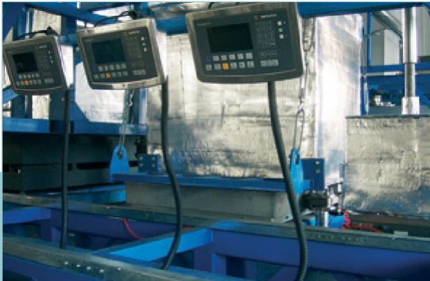
Combics 3 weight indicators' large displays provide excellent visible readout even in unfavourable conditions
