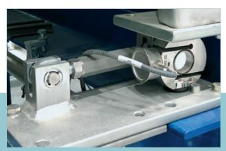
The S-type compression load cells under the additive container tanks provide highly precise measurement results
