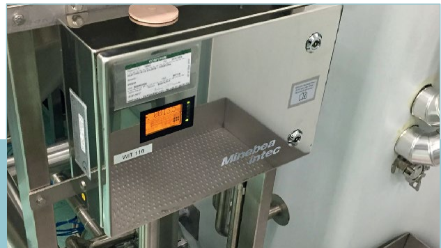
Minebea Intec's load cells and weighing electronics provide reliable weighing of process vessels
