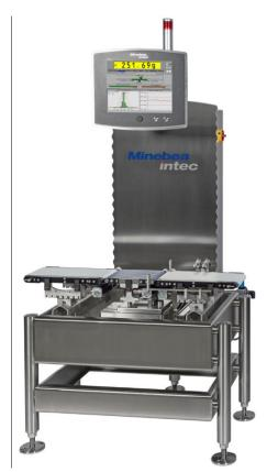
The new  ${\rm Flexus}^{\scriptscriptstyle (\! 9\!)}$  Highspeed from Minebea Intec offers processing speeds of up to 2.6 m/s
